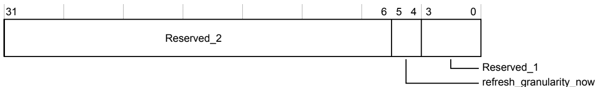
Figure 3-242 refresh_control_now register bit assignments
