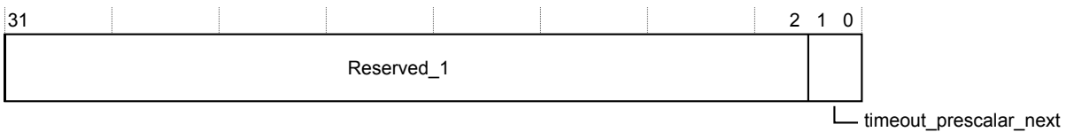
Figure 3-16 timeout_control_next register bit assignments
